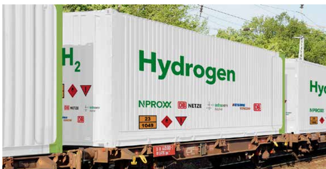
Figure 9.1: Cryogenic container capable of delivering “Green Hydrogen” to all points on the Iarnród Éireann Network (Image: Michael Ismar, NPROXX)
